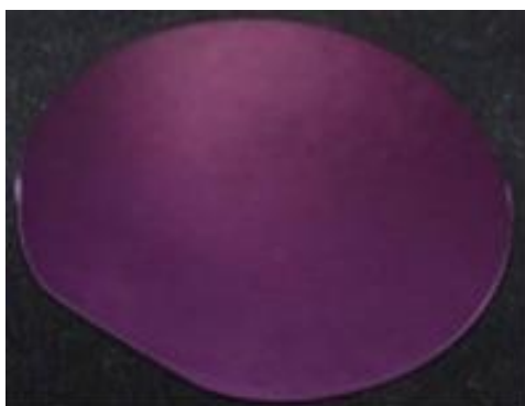
Figure 6: SiN film plasma deposited in a low-pressure plasma deposition process on a silicon wafer by application of a microwave-powered plasma array [4].
