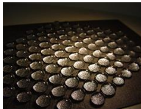
Figure 9: Originally completely hydrophobic surface of a gas diffusion layer (GDL), showing hydrophilic properties on the areas exposed to the plasma (cf. water droplets adhered to these hydrophilic areas after low-pressure microwave plasma treatment) [9-10].
