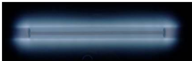
Figure 1: Axially homogeneous plasma formed around the Duo-Plasmaline low-pressure microwave plasma source [1].
