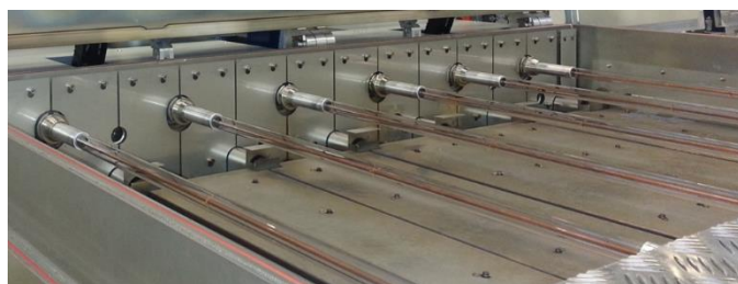
Figure 4: Plasma array consisting of six Duo-Plasmalines integrated into a process chamber for e.g. low-pressure plasma deposition of thin films used in the production of solar cells (courtesy of Meyer Burger Germany).
