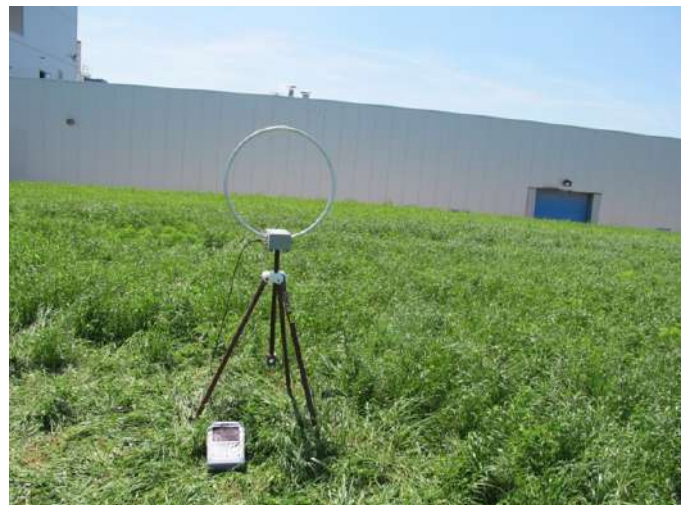
Fig. 4: Loop-antenna for the measurement at 27.12 MHz.
