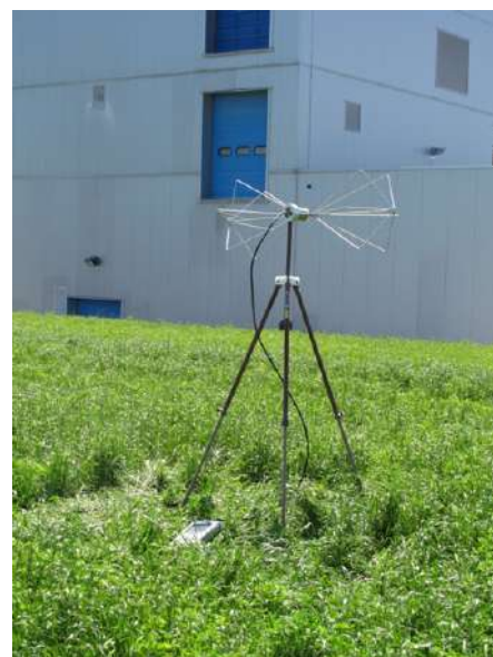
Fig. 5: Biconic antenna for measurement of harmonics between 50 MHz and 300 MHz.
